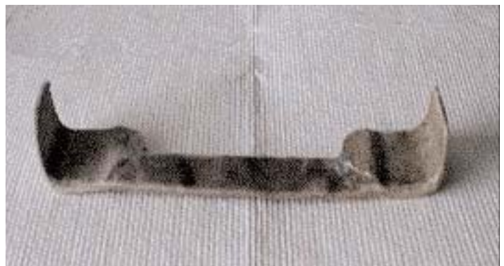
A car handle is an example of what has been made by Dr. Mohini Sain's lab when combining ultra-fine hemp fibre and bioplastics.
